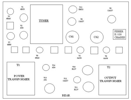
Figure 9. Chassis – diagram top view
